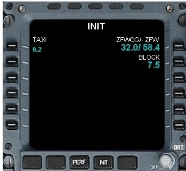
The MCDU PRESENTATION can be viewed as a reference for correct MCDU setup. The INIT A (TAXI, ZFWCG/ZFW and BLOCK entry) and PERF (FLAPS/THS entry) pages can be displayed.
