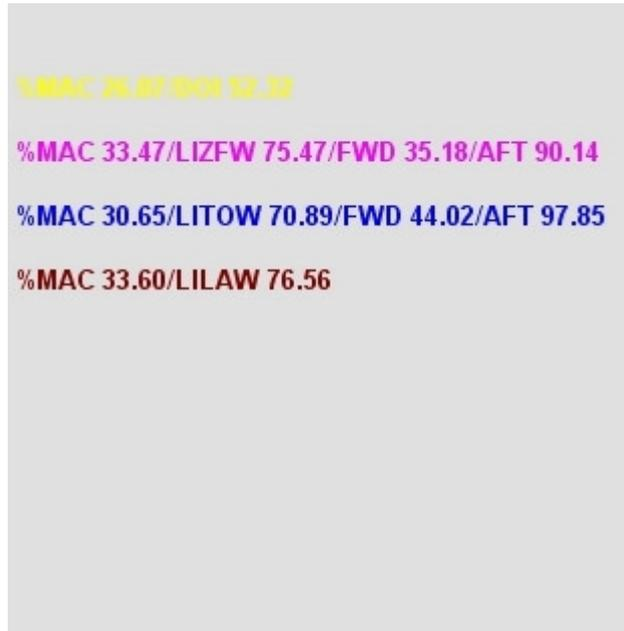
This section shows the detailed mathematical results of the actual aircraft loading for the various aircraft weights in terms of %MAC and LOAD INDICES (LI). The use of load indices is a mathematical method to calculate the passengers, cargo and fuel load of an aircraft.
