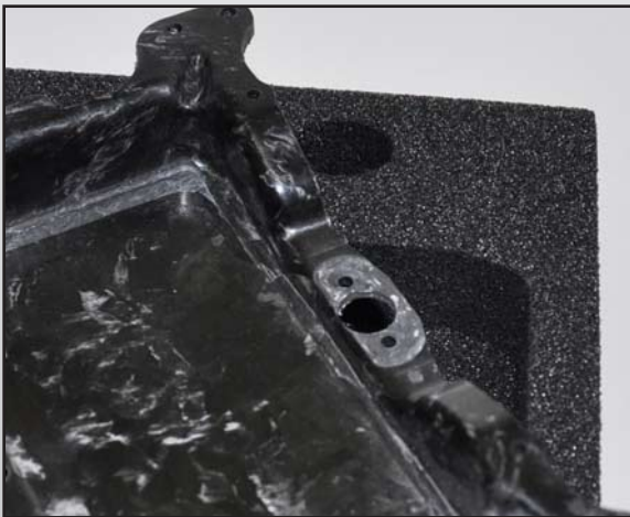
Front end, rear end and battery slot are CNC milled to ensure that everything is flat.
